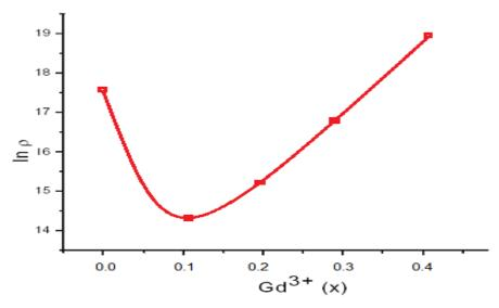
Fig.1. Variation of resistivity with concentration
