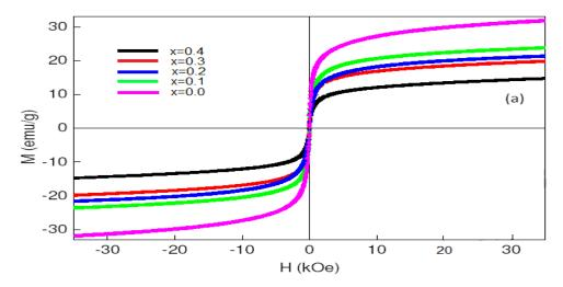
Fig.3. Hysterisis loop of  $NiGd_xFe_{2-x}O_4$  at different x (x=0, 0.1, 0.2, 0.3, 0.4)
